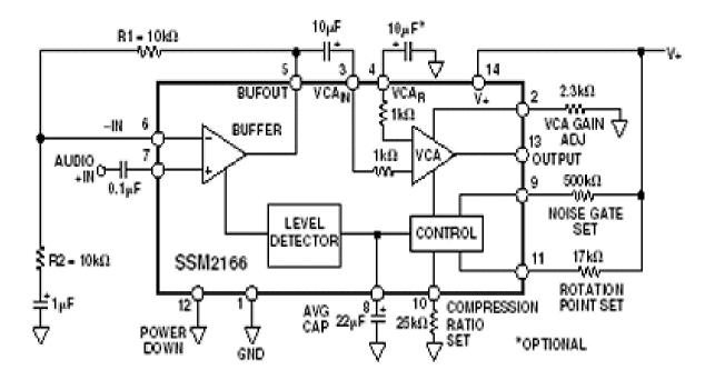
Figure 13: Functional Diagram
