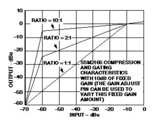
Figure 14: Compression and Gating Characteristics
