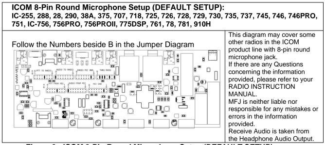
Figure 6: ICOM 8-Pin Round Microphone Setup (DEFAULT SETUP)
