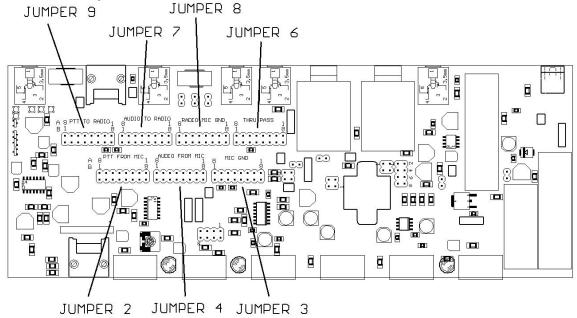
Figure 4: Internal Jumper Blocks
