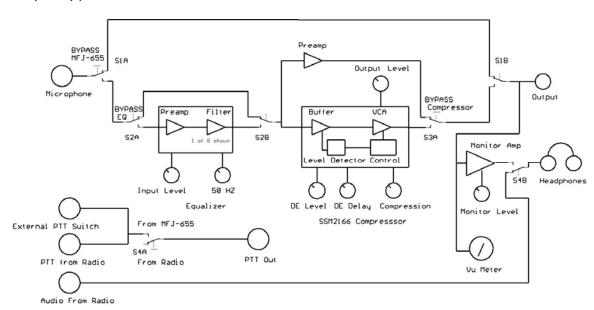
Figure 15: Block Diagram
